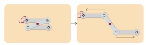
Toolboxes and scissor lifts use linkage mechanisms.
