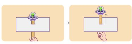
Door bolts and drawers use slider mechanisms.
